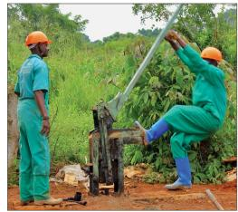
These special stabilized, interlocking soil bricks are dried in the fresh air and the sun, not fired in an oven. That means no one has to chop down a bunch of trees to make a fire for the brick oven. That saves a lot of trees and even reduces pollution.
